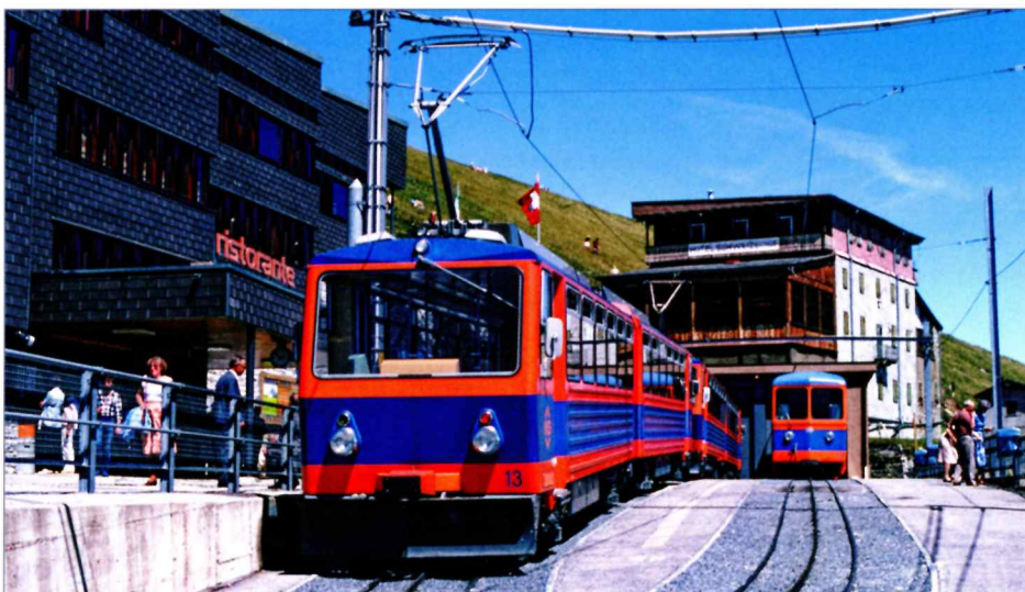
Generoso Vetta terminus on 8 August 1985. The summit hotel visible in the background has disappeared today, as has the summit restaurant of 1971 visible on the left, which is now replaced by the "Fiore di pietra". The two electric double railcars Bhe 4/8 Nos.13 and 12 and the diesel railcar Bhm 2/4 No.4 are waiting for passengers.
